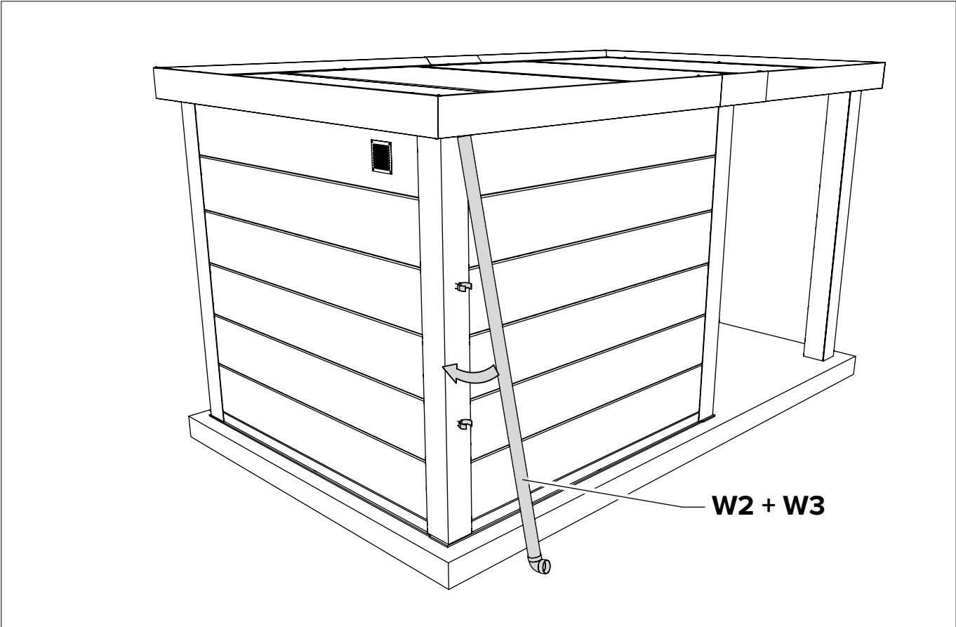
Drain / Afwatering / Drainage / Drainage
